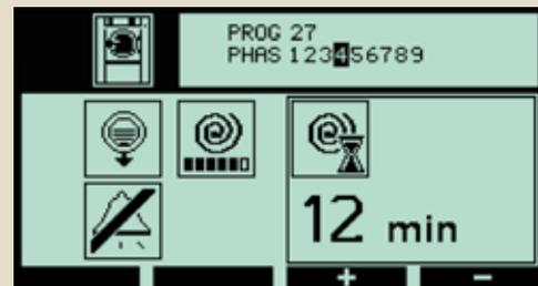
The Inteli screen indicates the operations being performed by the machine in each washing
