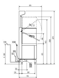
CWII Cold Water inlet 1 (cleaning) Drain
