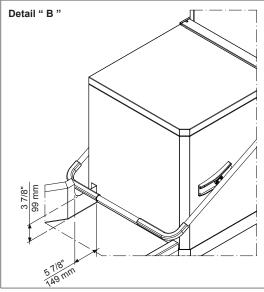
All tables must be connected to the dishwashing units according to local regulations and industry standards which may differ from the recommendations herein suggested. Electrolux Professional is not liable for any failure in complying with local design standards. Doc Nr: 59566BF00
